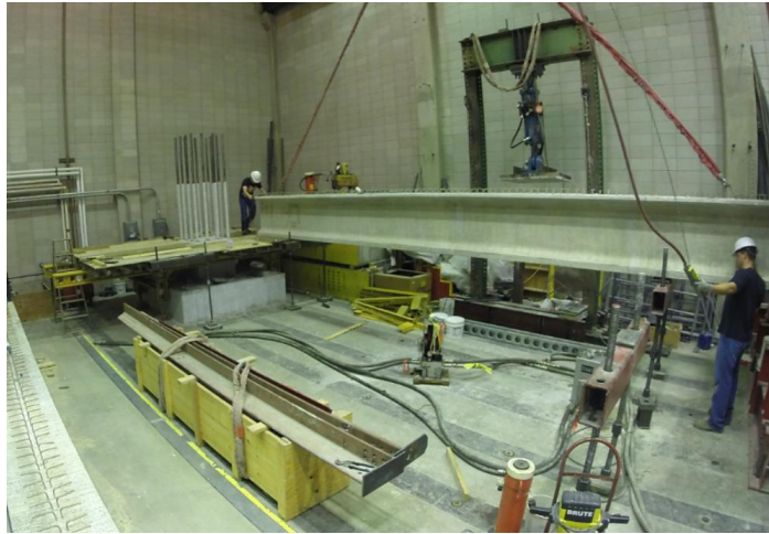
Figure 4-1 Place the Girder on Temporary Falsework
