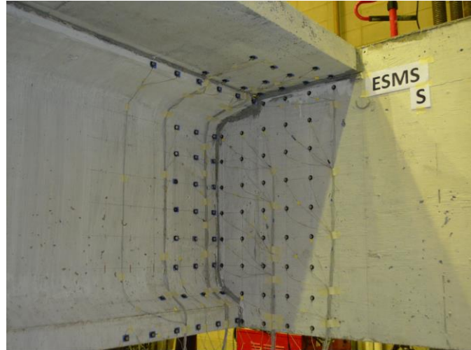
Figure 4-20 Optotrak System Marker Layout
